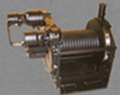
Sepdurance H200 motors out Planetary Gear Winch Line pull on bottom rope layer: 200-240 kN Rope length: 60 m
