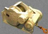
Sepmatic H100F Planetary Gear Winch Line pull on bottom rope layer: 100-120 kN Rope length: 60 m
